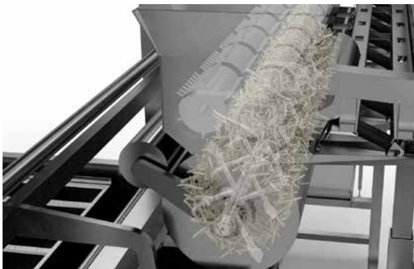
↳ Milling process: Mill rollers break down cheese loaves. The milled cheese falls into the mixing drum, where an agitator rotates. The drum's upper opening turns towards the salt station, where salt is added.
