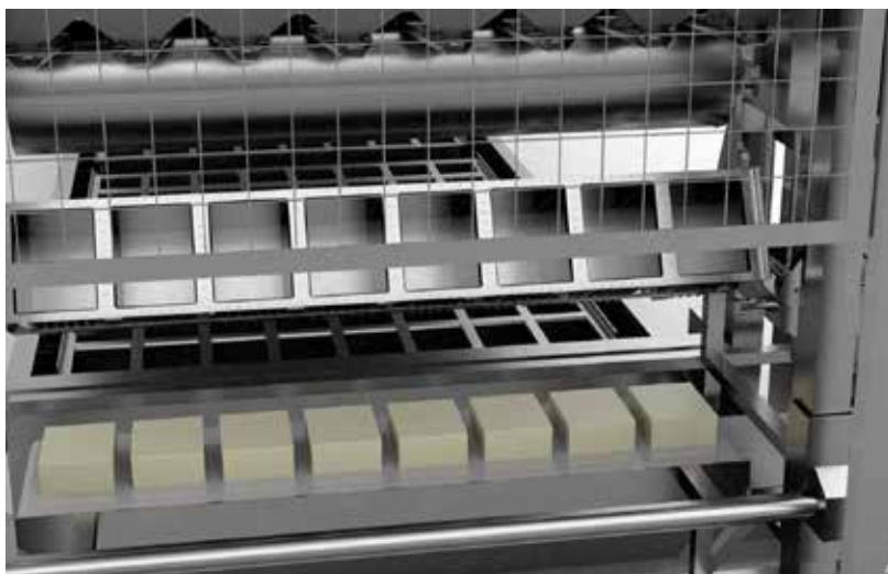
↳ De-molding and conveyor system: Pressed cheeses are turned and released onto a conveyor belt, ready for the next processing step.
